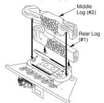
Figure 26 - Installing Rear and Middle Logs
